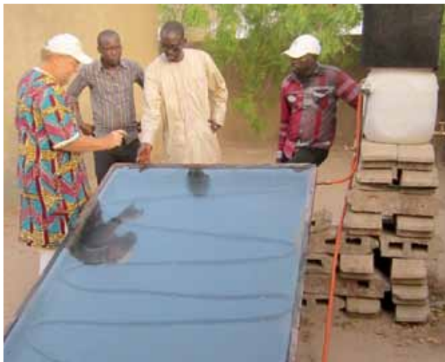
Barry Wheeler provides ongoing technical training to build the capacity of our field technicians. In 2015, he worked with the field team to engineer a low-tech passive solar water heater for the Gagnick Mack health post.
