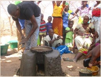
Once the walls are built up to just below the lip of the pot, participants can use water to smooth the sides of the walls. They should also ensure that the walls are straight and maintain a consistent width.
