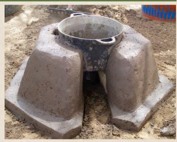
Next, participants should let the stove dry for three days. Three times a day, they should remove and twist the pot to ensure that the cookstove does not stick to the pot.
